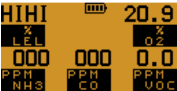
Display in alarm conditions
